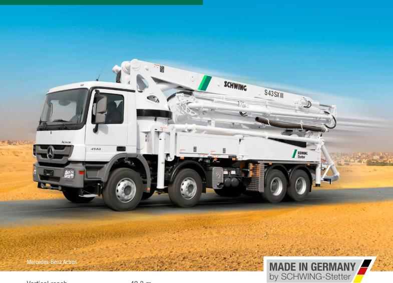
Vertical reach 42.3 m Concrete output max. 162 m³/h Pressure on concrete max. 85 bar
